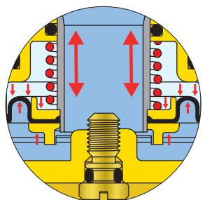
b) Device **(B)** regulates flow rate  $G$  by changing its bore cross section. The change in bore cross section determines hydraulic coefficient value ( $Kv$ ) of regulator device **(B)**, which remains constantly at:
