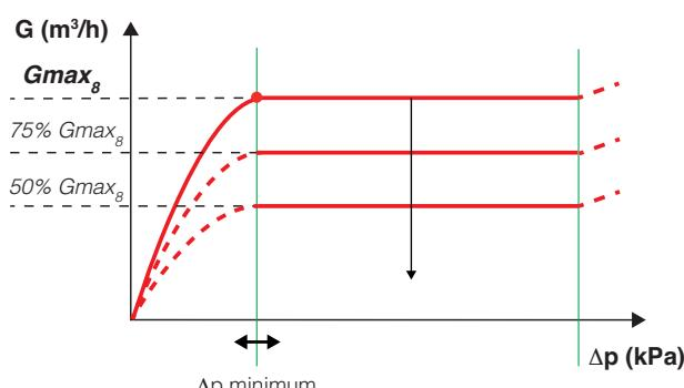
Turning the locking nut (10), which determines the number associated with the "Adjustment position", results in opening/closing of the bore cross section in the external obturator (13). Hence, each bore cross section set on the locking nut corresponds to a specific  $G_{max_x}$  value.
