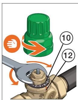
with a hexagonal key. The locking nut is fixed to a 10-position graduated scale, divided into steps corresponding to 1/10 of the maximum available flow rate, which is also shown on the scale (11). Turn the locking nut to the numerical position corresponding to the required flow rate (design flow rate), referring to the "Flow rate adjustment table". The notch (12) on the valve body is the physical positioning reference.
